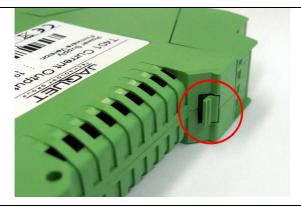
To open press both fastening clips together and pull out at the same time the upper side of the housing.
