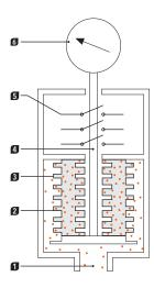
The density monitors are filled at works to the customer's gas density specification (variant with three micro switches is shown).
